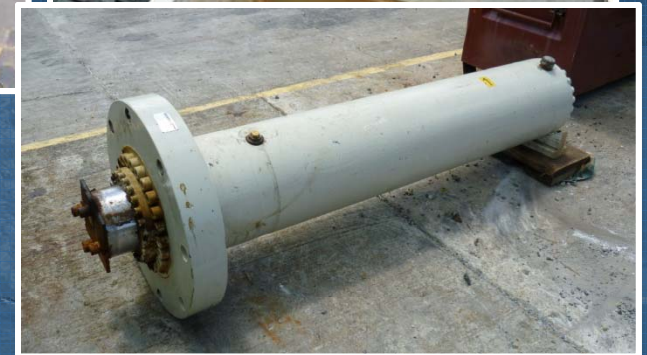
1 prototype cylinder brought to failure.
