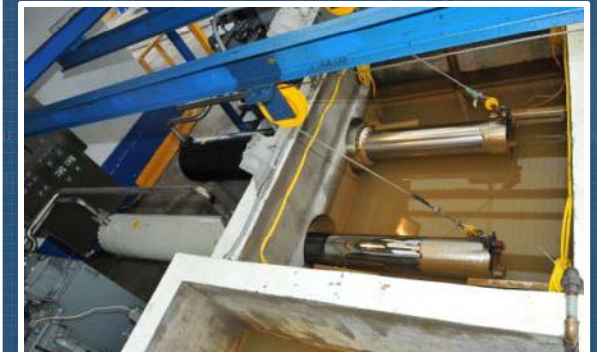
Testing 4 prototype cylinders in 2 tanks
